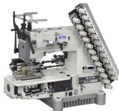
UN008-12064P/VSQ/VSM 多针双链式环缝机 (下松紧线缩褶打缆) Multi-needle double-chain circular sewing machine (Bottom elastic shirring) (Elastic down/general thread up smocking)
